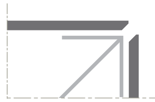
Figure 5: Mitred External Corner Detail
